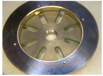
and two plunge cuts made at 90 degrees to the face with a 90 degree tool to form the two grooves. A large round nosed tool was then used to form the decora-
